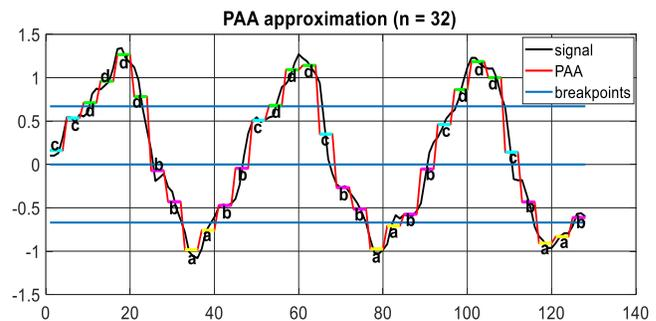
Figure 1. Processed signal, PAA technique, breakpoint lines that define ranges of values, and finally, the symbols are illustrated all together.
