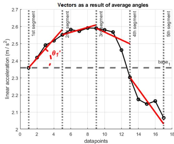
Figure 3. Every segment of the time series is replaced with a vector that has its initial point at the first point of the segment and forms an angle with the horizontal axis equal to  $\theta_i'$ . Red lines are the slope approximations, and the continuous black line is the signal.
