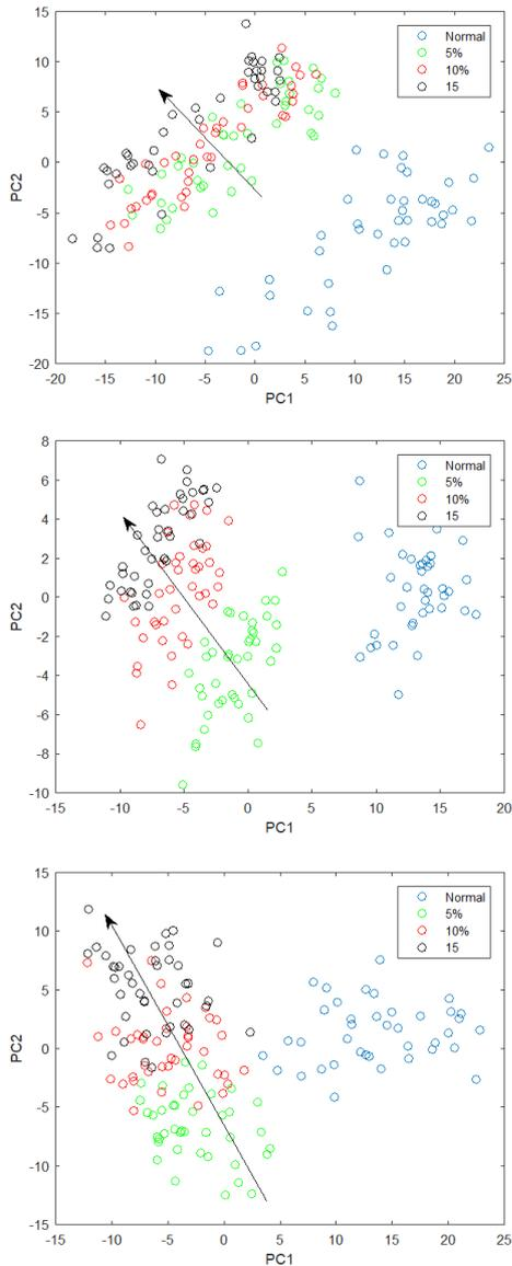
Fig. 4: Projection of the features up to 1 kHz to a 2 dimensional space (from top to bottom: current, commercial flux measurement, custom made probe flux measurement).
