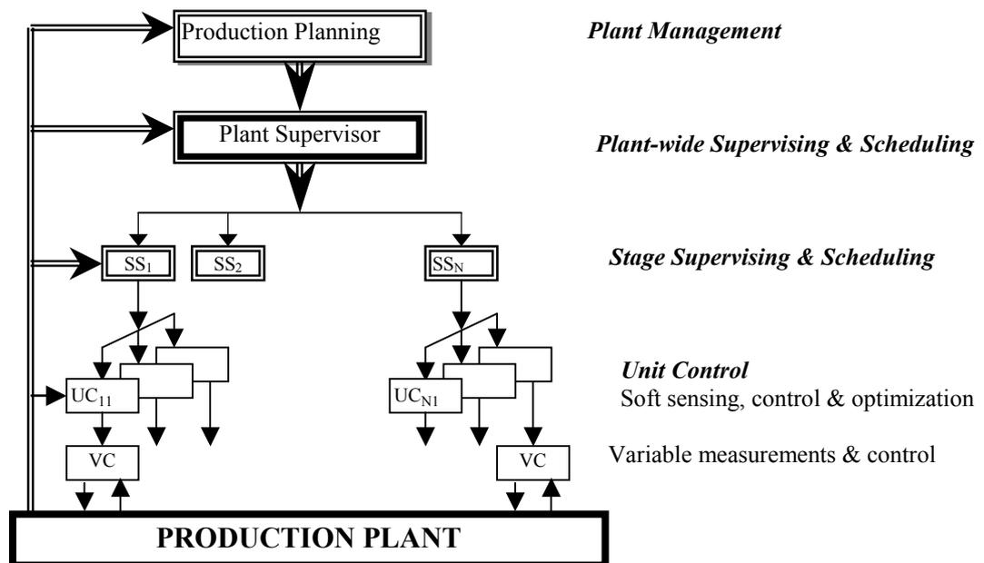
Figure 1. Hierarchical integrated control system
