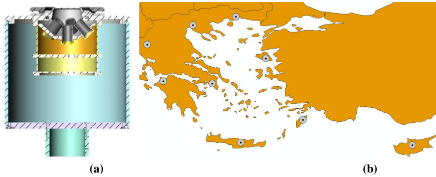
Fig. 4. a) Schematic representation of the actinometers used for measurements in the UV spectrum. b) The UV network (gray dots).
